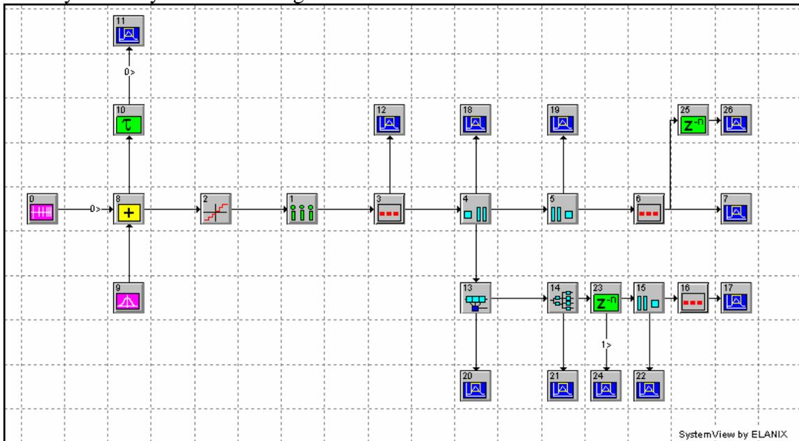
Note that there is a delay, Token 23, that is required for the bits-to-symbol converter to work. The function of this delay is to align the 8-bit sequences in the bit stream out of the decoder with what is required by the bit-to-symbol decoder, which simply counts from the first symbol.
